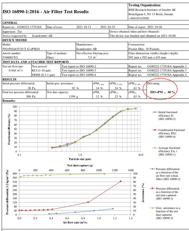
NOTE: The results of this test relate only to the test device in the condition stated herein. The performance results cannot by themselves be quantitatively applied to predict filtration performance in all "real life" environments.
